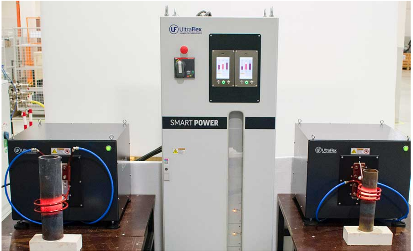
Fig. 3. Modular power supply with two separate outputs
