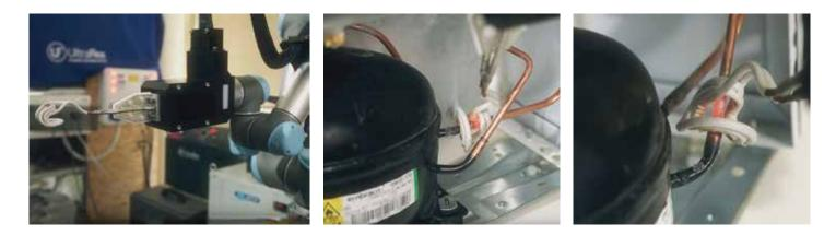
Dragon 15 integrates the Ultraflex W15 (15 kW) induction heating system with a Universal Robots cobot (UR 5) to achieve a fully automated brazing process. The system has been successfully used to replace the outdated and unsafe torch brazing widely used in the industry.
