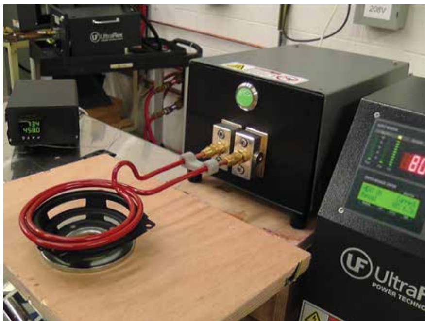
3. Setup of Induction System with Speaker Basket.
