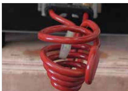
2. The aluminum sample levitated in the coil by induction.
