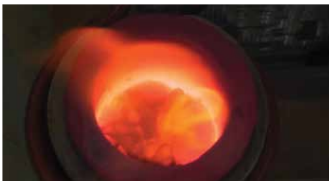
3. As the temperature increases, the dental scrap starts to melt.
