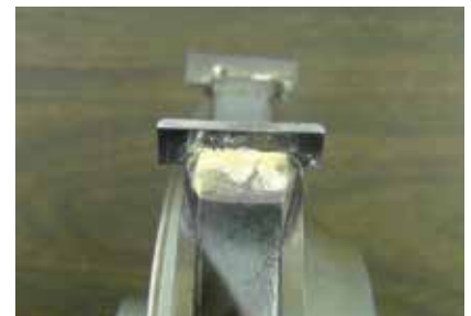
3. Resulting re-braze repair
