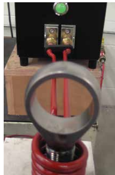
3. Induction Coil is placed inside Steel Tube
