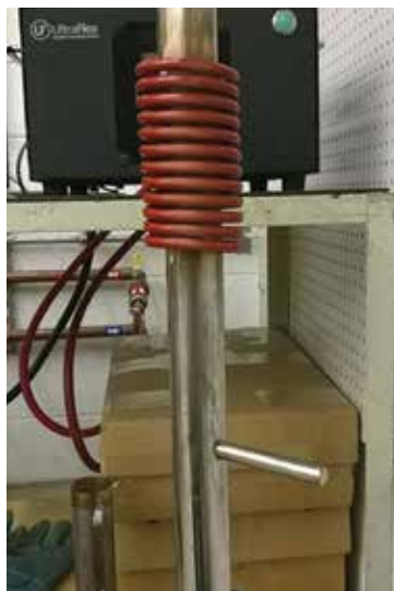
2. Stainless Steel tube heated with UPT-S5
