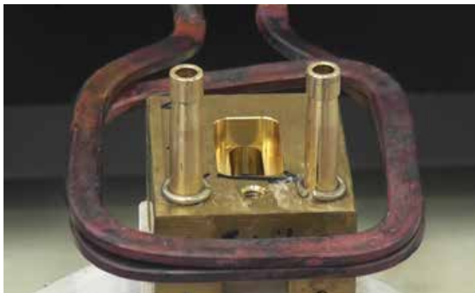
1. Braze Brass Fittings into Brass Housing: the barb fittings are positioned into the housing, with a preform placed at the position of the joint. The assembly is then positioned into the induction coil.
