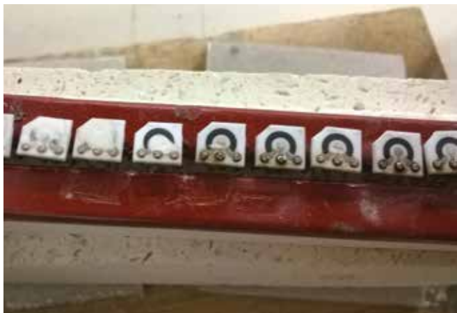
1. The small PCB sub-assemblies are positioned in the induction coil. Preliminary testing showed that pins heated best when positioned above the coil. Tempilaq, a temperature monitoring paint, is painted onto the pins, so we can monitor their temperature.
