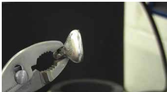
6. The metal is separated from the slag, which is the waste materials from the scrap.
