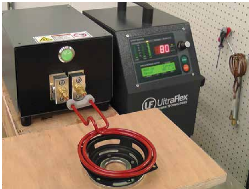
2. Setup of Induction System with Speaker Basket.
