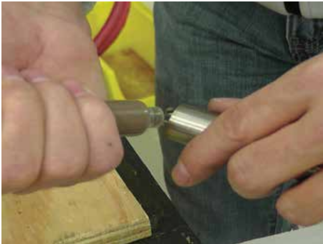
1. Brazing flux is applied
