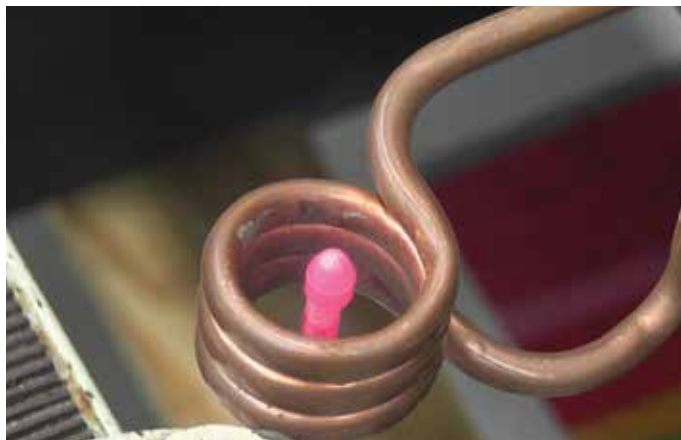
3. In-process picture of Test 3, with the bullet-shaped carbide heating using UPT-S5 5 kW Induction System.
