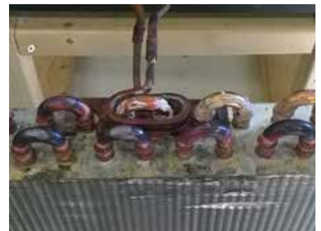
3. We braze each u-shaped return. Brazing takes approximately 35 seconds per return.
