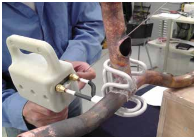
2. UBraze is positioned at the joint.
