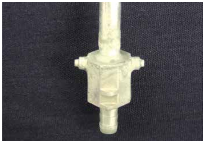
4. The completed aluminum to aluminum Braze.
