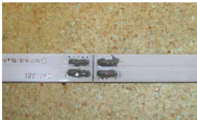
1. Solder paste is applied to the pads.
