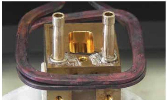
2. Braze Brass Fittings into Brass Housing: after approximately 30 seconds.
