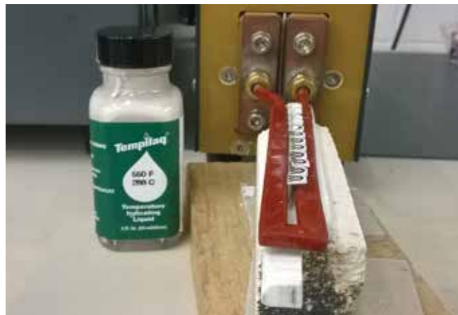
2. Another view of the small PCB sub-assemblies positioned in the coil.
