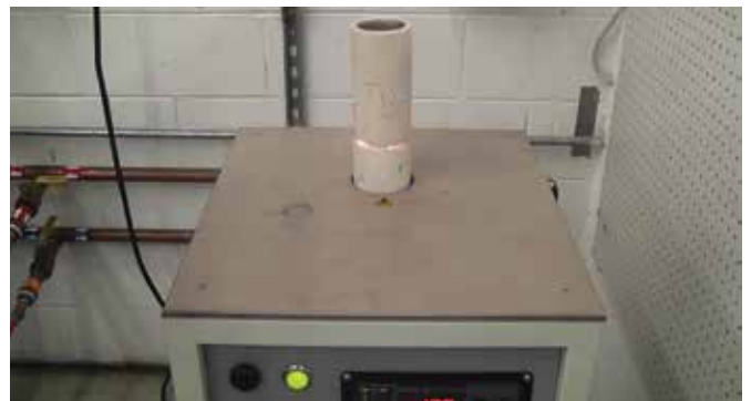
2. Here we see the second crucible used as a lid for the primary crucible.
