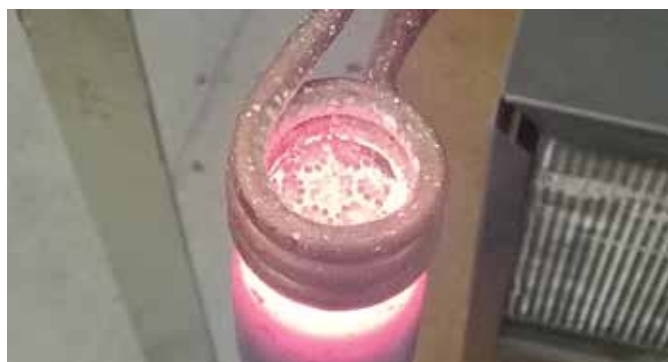
3. Hot forming steel cable application test: The steel cable heats in the induction coil.
