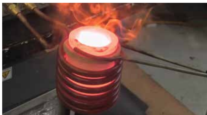
4. Once completely molten, the crucible is carefully removed from the coil using tongs.
