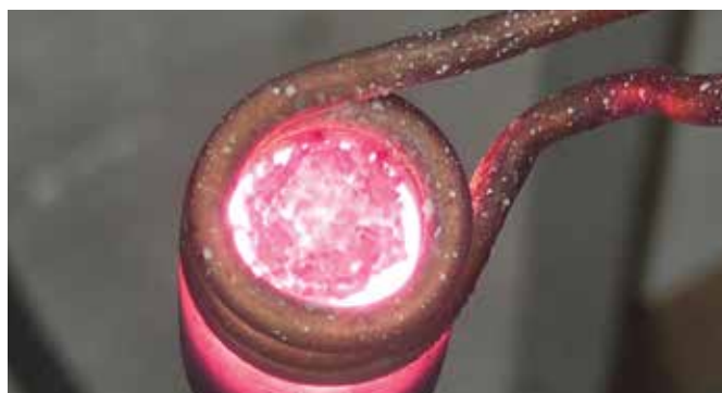
4. Hot forming steel cable application test: The end of a steel cable is heated to 2000°F (1093°C).
