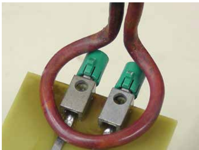
3. Induction Coil is placed above the components.
