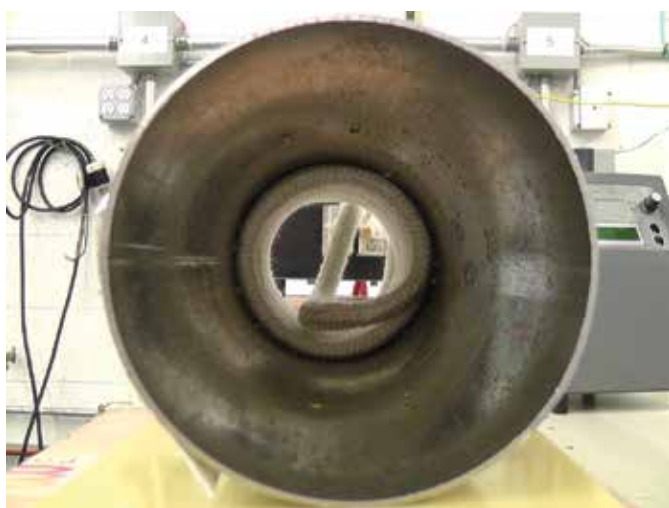
3. Induction preheat steel tubing
