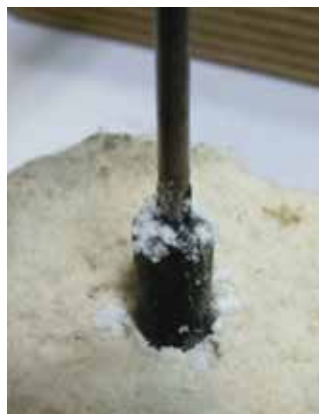
2. Brazing paste and flux are placed on the assembly
