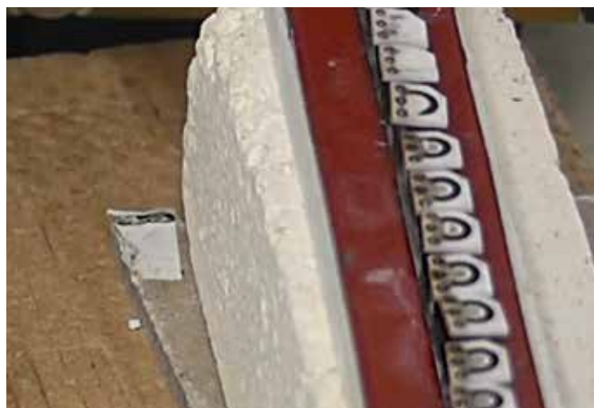
4. Here we see at the end of the heating cycle that the tempilaq paint has changed color, indicating that we have reached the target temperature of 500F. The test results show we can heat at the rate of 1 PCB assembly every 0.3 seconds, which exceeds the target of 1 second per PCB. By using UPT-SB3/1000 system, the customer's production rates can grow to meet increasing demand for the parts.
