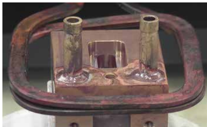
7. Braze Brass Fittings into Brass Housing; after approximately 2:30. The finished braze, showing a consistent fillet at the braze joint.
