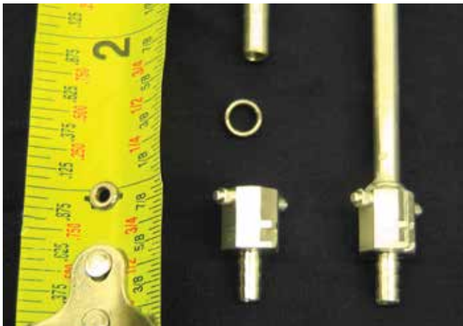
3. The aluminum tubing and aluminum component to be brazed, shown separately and as assembled.
