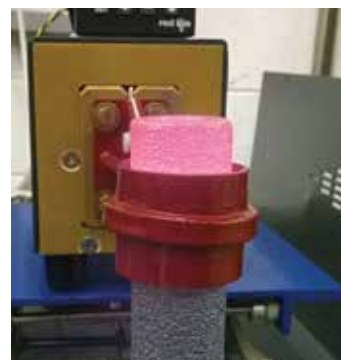
3. Silicon Carbide Cylinder heated to 2700-2800°F with 1 MHz induction
