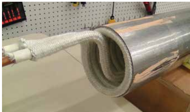
2. Induction Coil is placed inside Steel Tube
