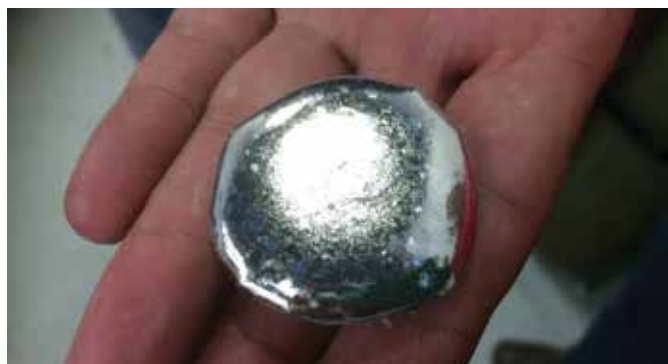
7. The final melted piece of platinum after cooling.
