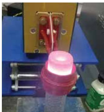
2. Silicon Carbide Cylinder heated to 2700-2800°F with 1 MHz induction.
