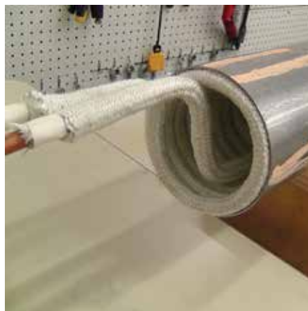
Induction Coil is placed inside Steel Tube
