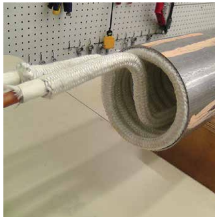
Induction Coil is placed inside Steel Tube
