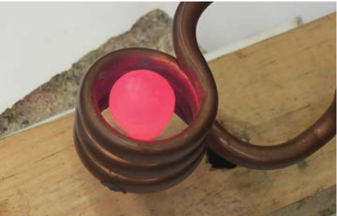
2. In-process picture of Test 2, with the spherical carbide heating using UPT-S5 5 kW Induction System.
