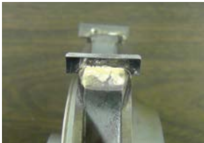
3. Resulting re-braze repair
