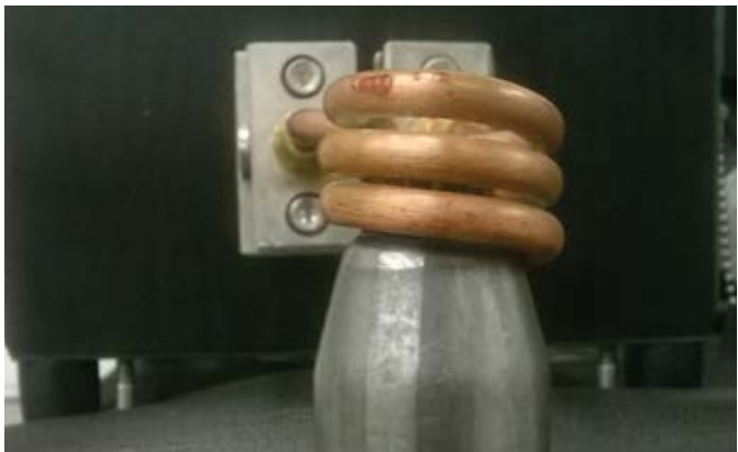
1. Hot forming steel cable application test: The steel cable with attached ferrule is positioned in the induction coil. No part of the load is to touch the coil.
