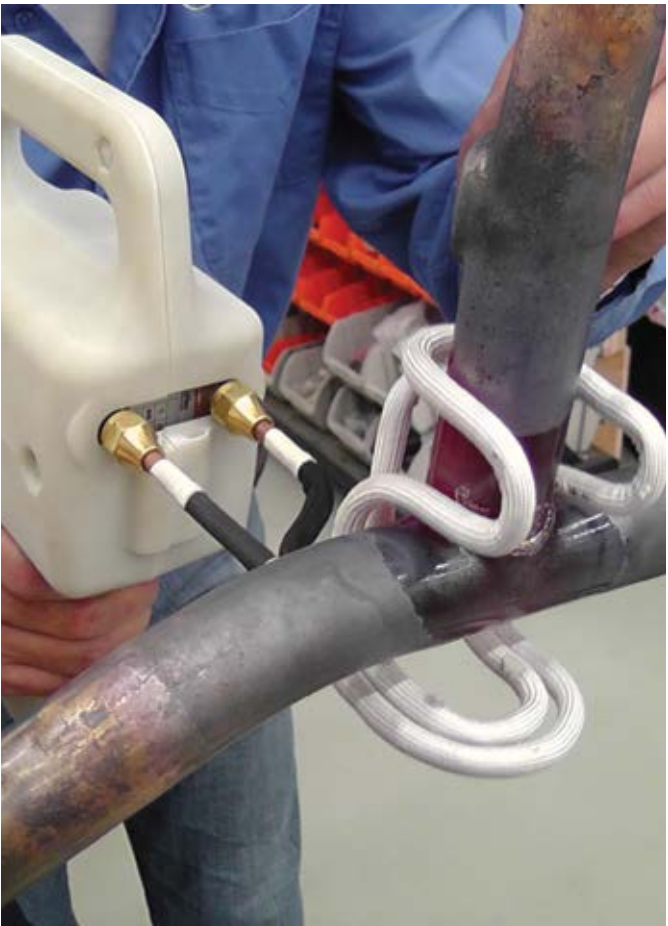
5. The UBraze is re-positioned on the other side of the joint, to heat the area previously left open by the T Coil.
