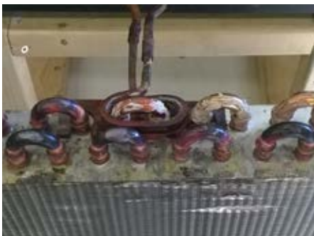
3. We braze each u-shaped return. Brazing takes approximately 35 seconds per return.
