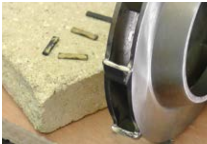
1. Photo showing the area following carbide removal
