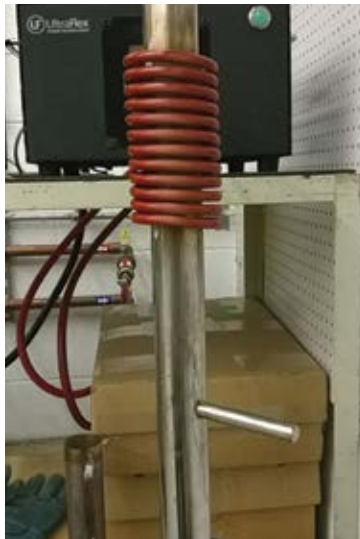
2. Stainless Steel tube heated with UPT-S5
