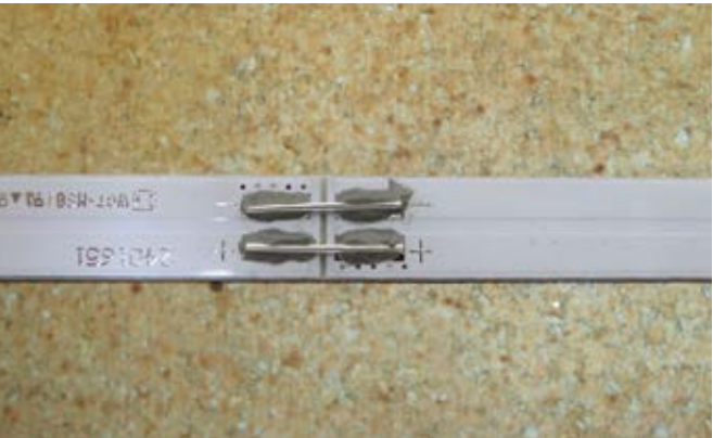
2. Jumpers are placed in the solder paste across the pads of the adjacent PCBs.
