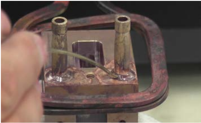
6. Braze Brass Fittings into Brass Housing: after approximately 2:15. A small amount of brazing alloy is added by hand during the heating, to fill the opening not covered by the preform.
