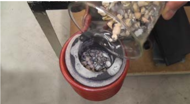
1. Flux and Dental Scrap are added to the crucible, which is positioned in the induction coil.
