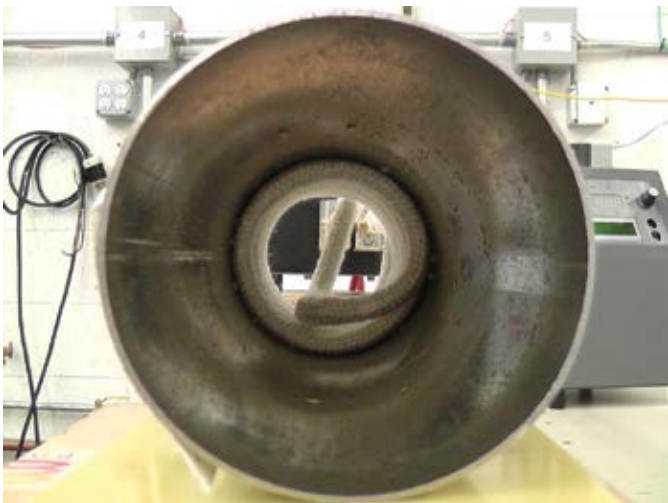
3. Induction preheat steel tubing
