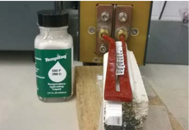
2. Another view of the small PCB sub-assemblies positioned in the coil.
