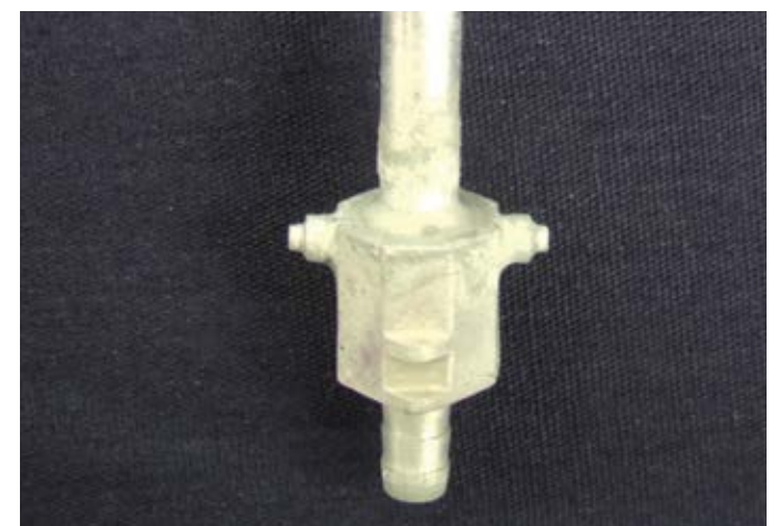
4. The completed Aluminum to Aluminum Braze.
