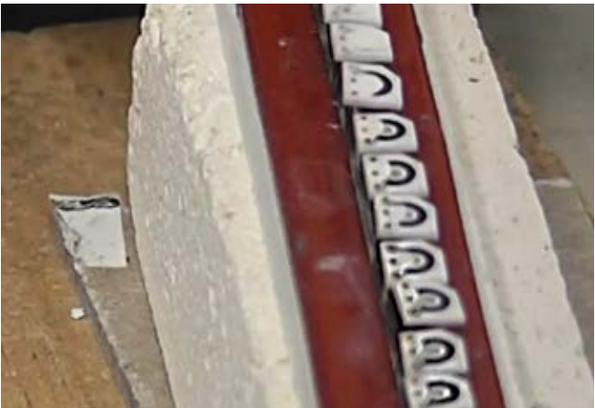
3. This close-up view shows the small PCB sub-assemblies at the beginning of the heating cycle.
