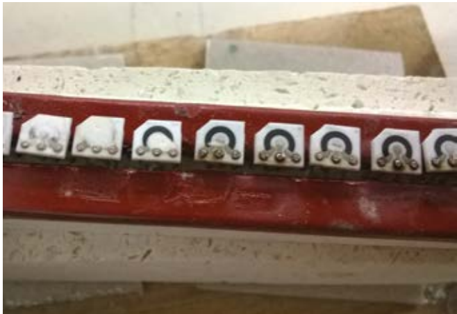
1. 1. The small PCB sub-assemblies are positioned in the induction coil. Preliminary testing showed that pins heated best when positioned above the coil. Tempilaq, a temperature monitoring paint, is painted onto the pins, so we can monitor their temperature.
