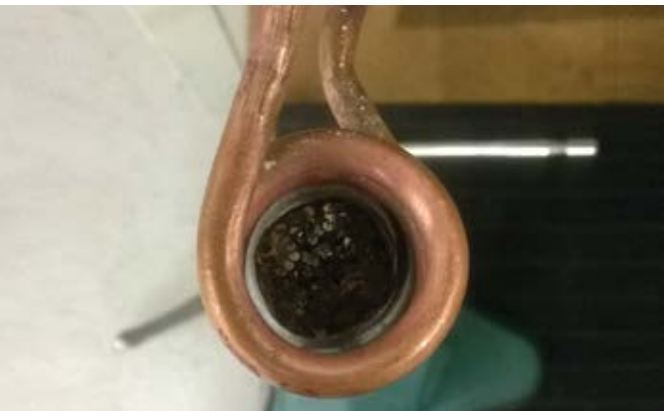
2. Hot forming steel cable application test: Top View of the steel cable positioned in the coil.
