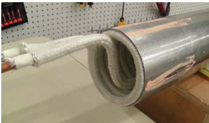
2. Induction Coil is placed inside Steel Tube
