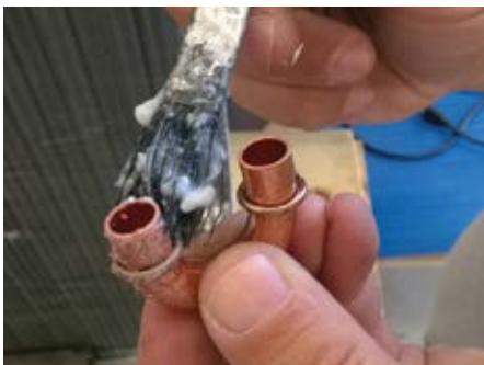
1. Flux is applied to the "U"-shaped returns
