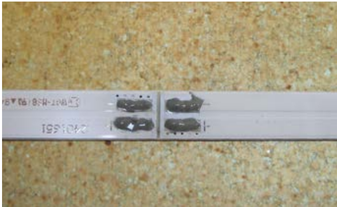
1. Solder paste is applied to the pads.
