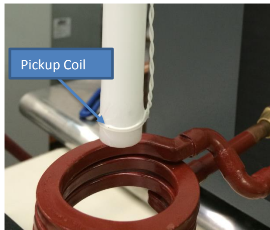
Figure 8: Pickup Coil used for Measurements
