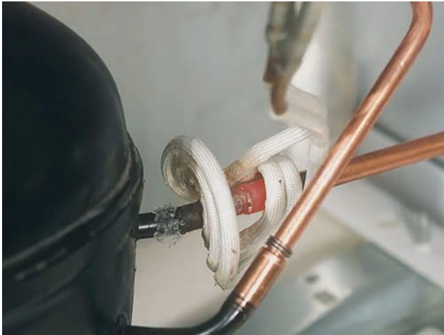
Fig. 2. Induction brazing in a refrigerator assembly
