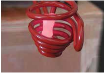
3. The melted aluminum at the end of the process, stably contained by levitation.
