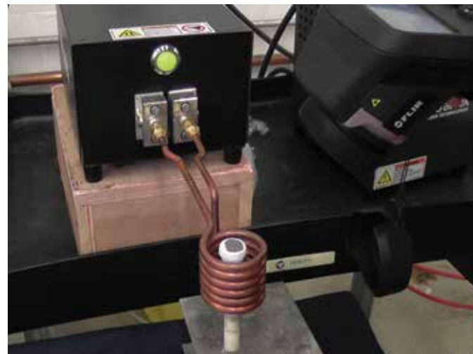
1. Vial has been placed into the coil. An Infrared Camera is positioned above to measure the temperature.
