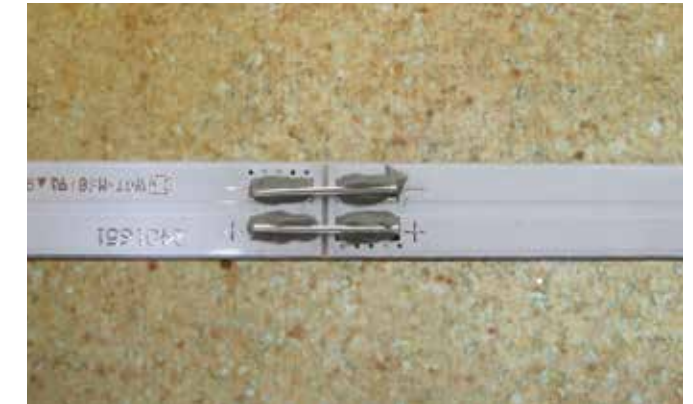
2. Jumpers are placed in the solder paste across the pads of the adjacent PCBs.
