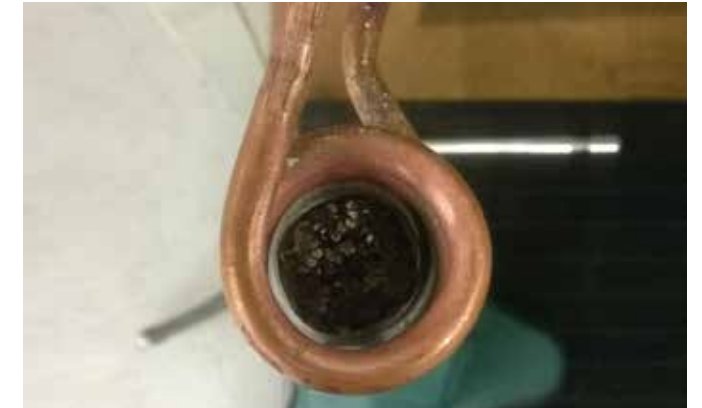
2. Top view of the steel cable positioned in the coil.
