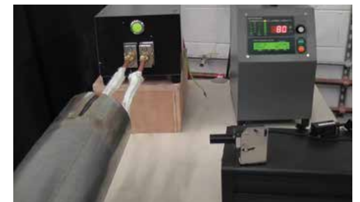
6. Tempilaq and Infrared temperature monitor are used to verify when we have reached 700F.
