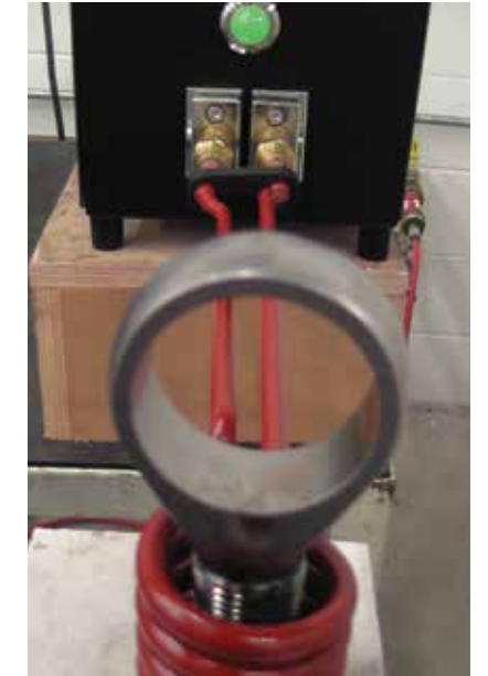
3. Induction Coil is placed inside Steel Tube
