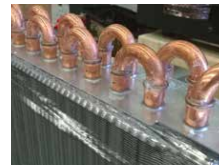
2. "U"-shaped returns are assembled to the receiving tubes.
