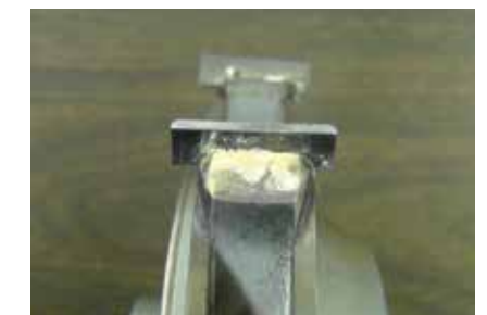
3. Resulting re-braze repair
