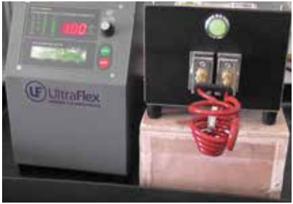
1. UPT-S2 power supply, HS-4 heat station, and levitating sample at the beginning of operation.
