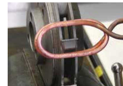
2. Position of the part for the heat-cycle to remove the used carbide – heat time test 8 seconds
