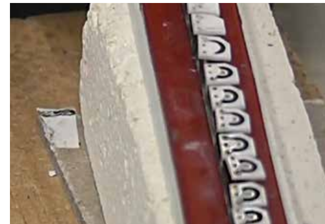
3. This close-up view shows the small PCB sub-assemblies at the beginning of the heating cycle.
