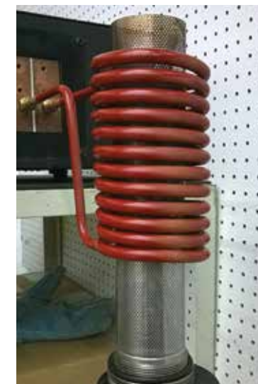
2. Mesh Tube tested with UPT-S5 Induction Heating System for Plasma Research.
