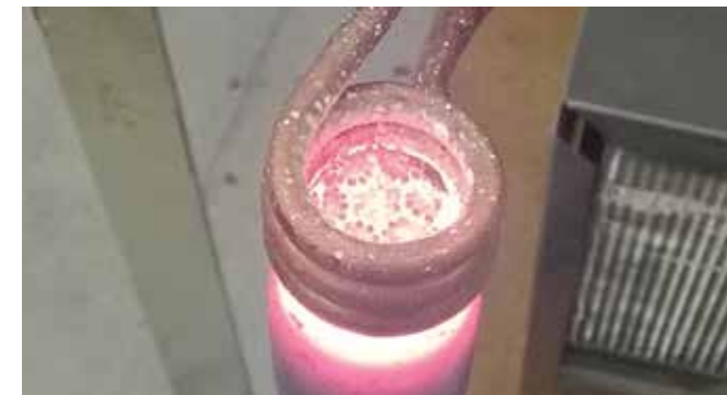
3. The steel cable heats in the induction coil.
