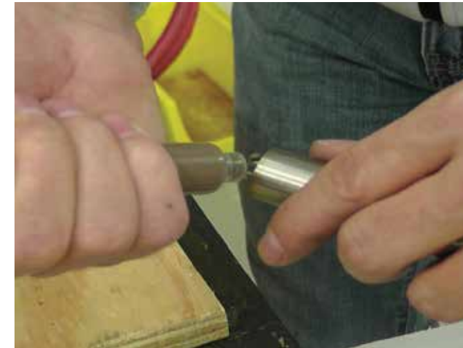
1. Brazing flux is applied
