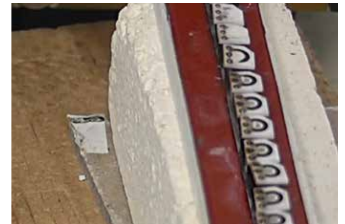
4. Here we see at the end of the heating cycle that the tempilaq paint has changed color, indicating that we have reached the target temperature of 500F. The test results show we can heat at the rate of 1 PCB assembly every 0.3 seconds, which exceeds the target of 1 second per PCB. By using UPT-SB3/1000 system, the customer's production rates can grow to meet increasing demand for the parts.
