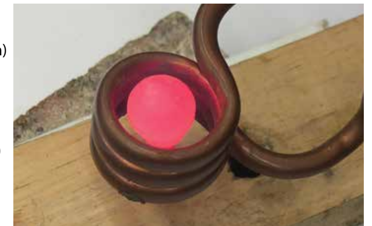
2. In-process picture of Test 2, with the spherical carbide heating using UPT-S5 5 kW Induction System.
