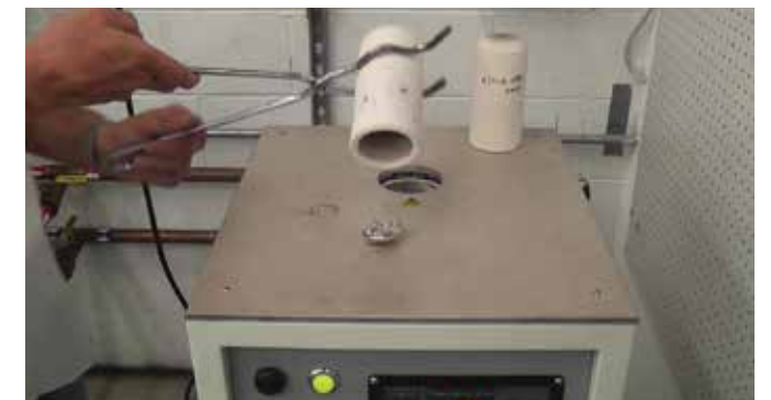
6. After cooling time, the platinum releases from the crucible.
