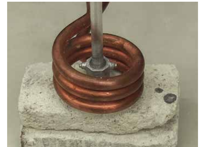
2. Power was turned off after 14 seconds, and the process of brazing aluminum to aluminum was complete.
