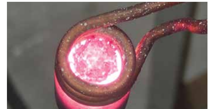
4. The end of a steel cable is heated to 2000°F (1093°C).
