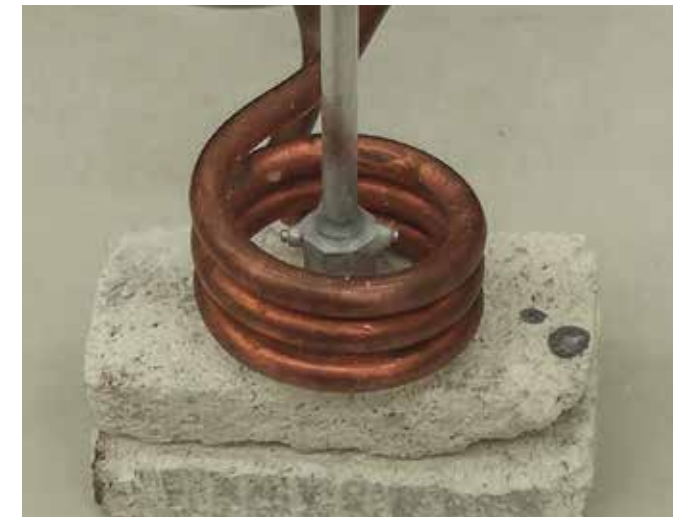
1. The aluminum component and aluminum tubing were assembled together with the alloy ring. Flux was added. The part was positioned in the induction coil.
