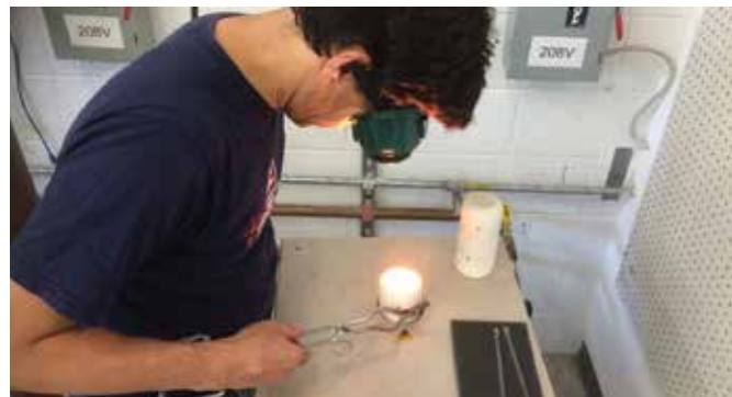
1. During the test, the engineer taps periodically on the crucible to help in the heating process. The engineer is wearing welding goggles, due to the brightness of the molten platinum.
