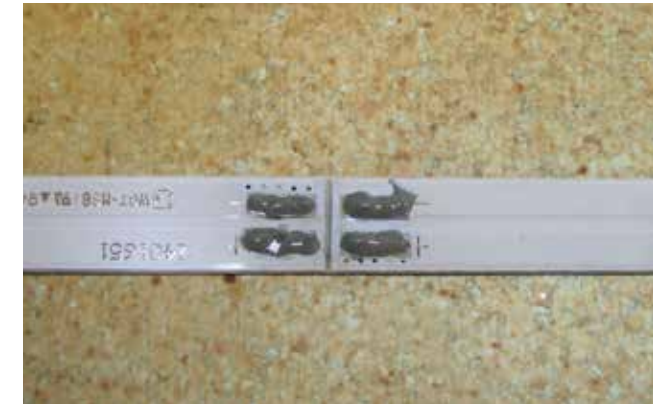
1. Solder paste is applied to the pads.
