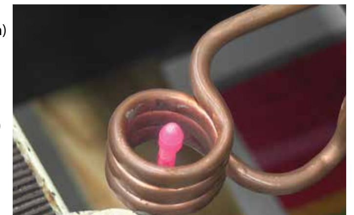
3. In-process picture of Test 3, with the bullet-shaped carbide heating using UPT-S5 5 kW Induction System.
