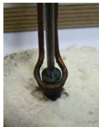
1. The assembly is positioned on refractory support.
