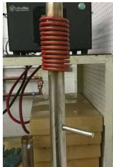
2. Stainless Steel tube heated with UPT-S5
