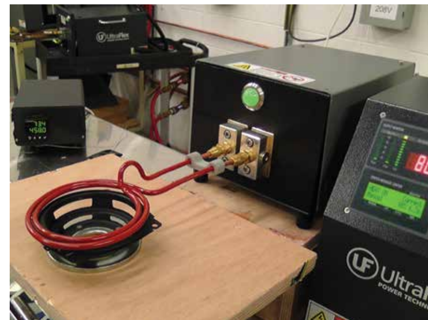
3. Setup of Induction System with Speaker Basket.
