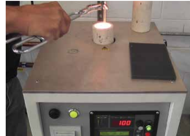
3. During test 2 a pipette was lowered into the molten platinum to take a sample.
