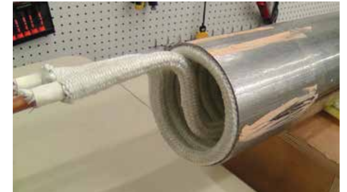
2. Induction Coil is placed inside Steel Tube
