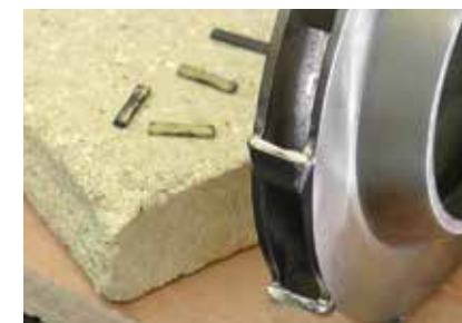
1. Photo showing the area following carbide removal
