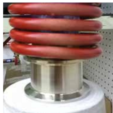
2. Mesh Tube tested with UPT-S5 Induction Heating System for Plasma Research.
