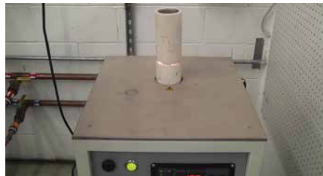
2. Here we see the second crucible used as a lid for the primary crucible.
