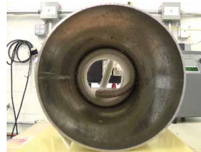
3. Induction preheat steel tubing
