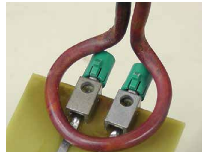
3. Induction Coil is placed above the components.
