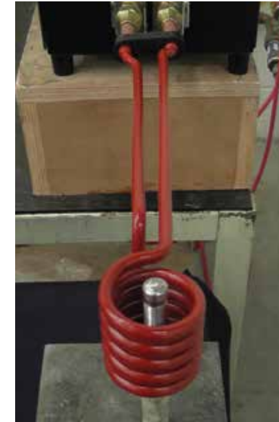
1. UPT-S5, HS-4 and Induction Coil are set up
