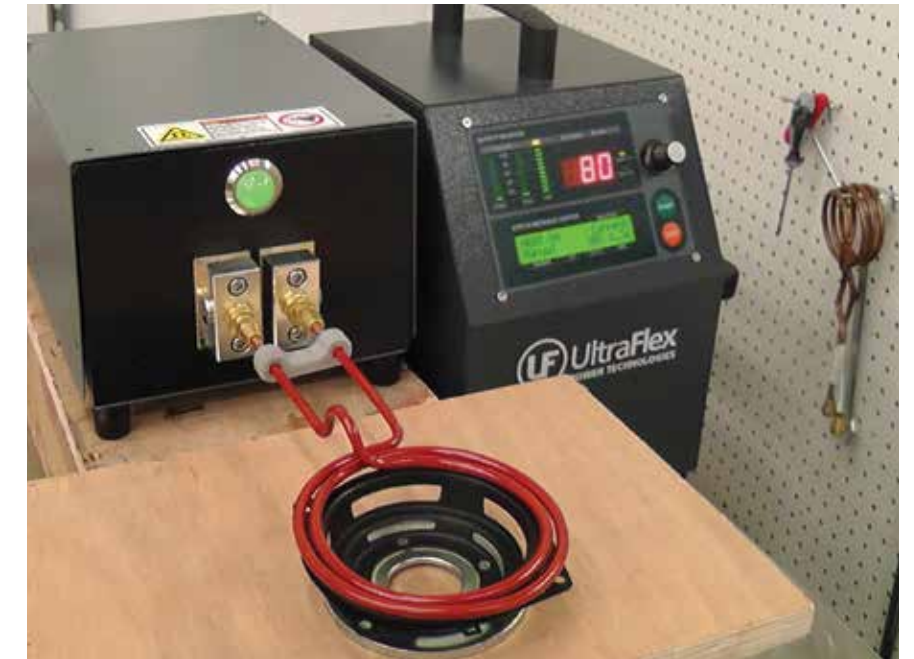
2. Setup of Induction System with Speaker Basket.
