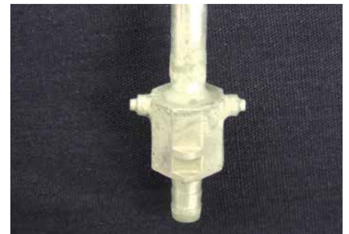
4. The completed aluminum to aluminum braze.
