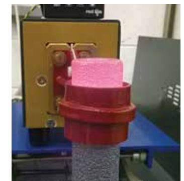
3. Silicon Carbide Cylinder heated to 2700-2800°F with 1 MHz induction
