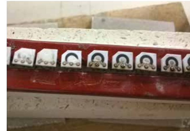
1. The small PCB sub-assemblies are positioned in the induction coil. Preliminary testing showed that pins heated best when positioned above the coil. Tempilaq, a temperature monitoring paint, is painted onto the pins, so we can monitor their temperature.
