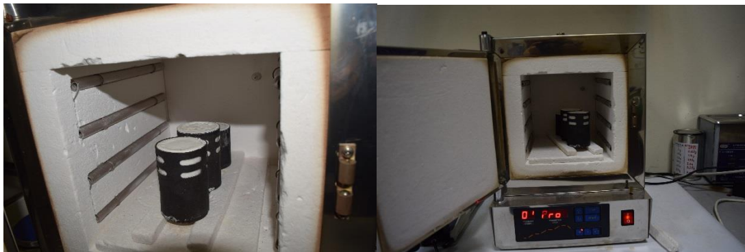
Fig. 12 - Placing the investment in the burnout oven
