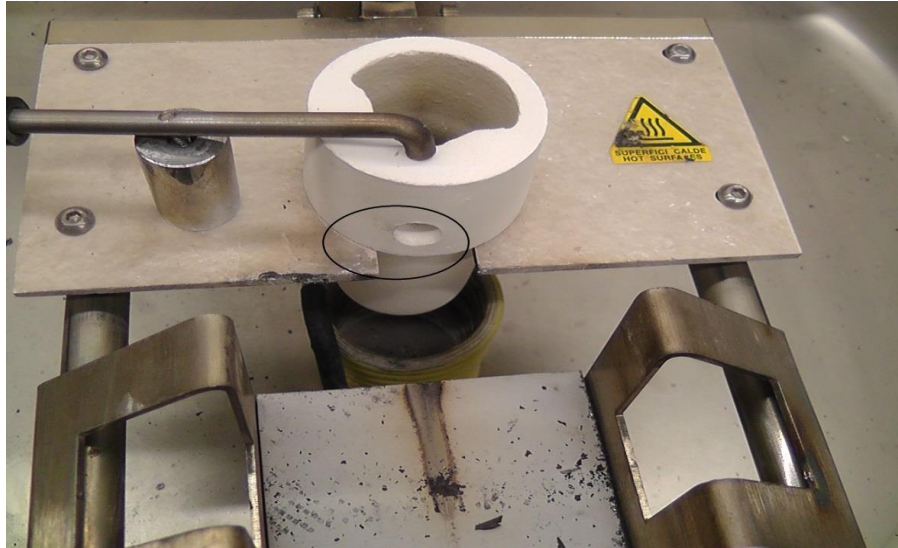
Figure 12: placing the crucible in the plate
