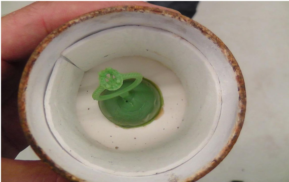
Figure 5: spacing the ring from the flask
