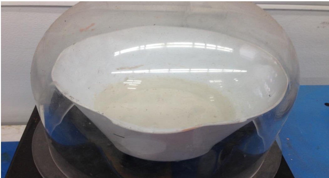
Figure 7: mixing platinum investment under vacuum
