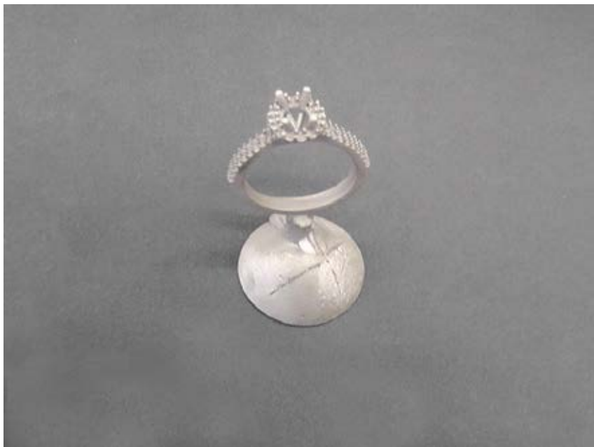
Figure 16: A different ring after a completed cast
