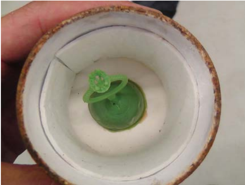
Figure 5: spacing the ring from the flask
