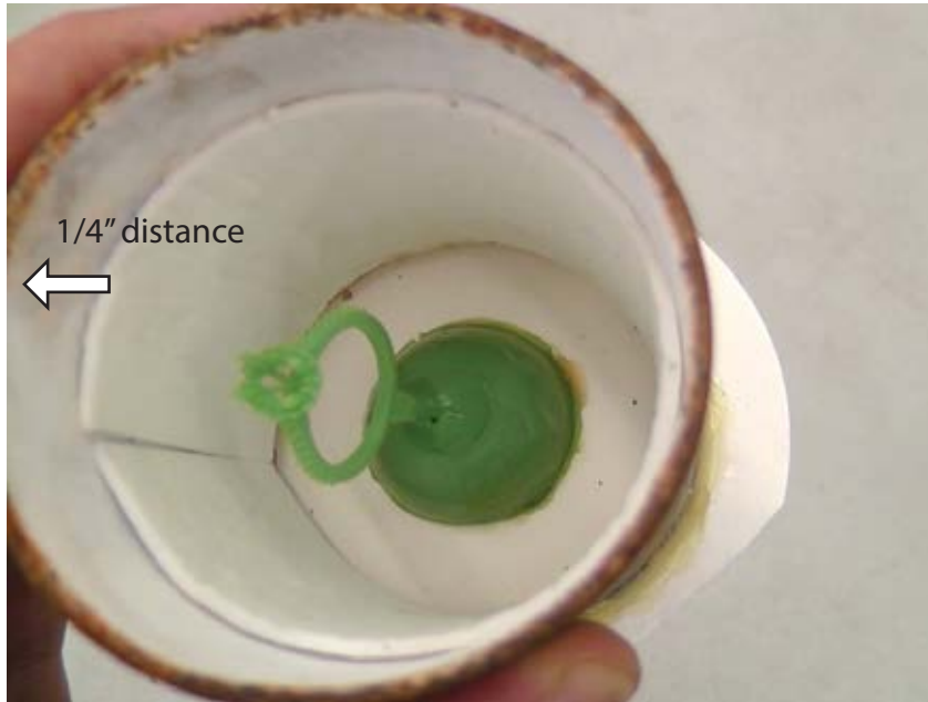
Figure 3: placing the liner paper into the metal flask
