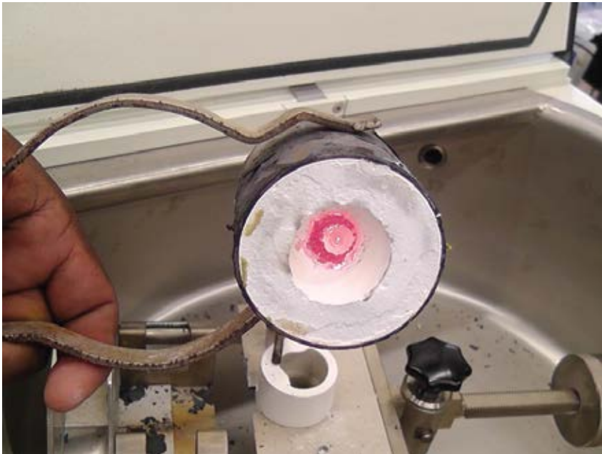
Figure 13: A flask after casting
