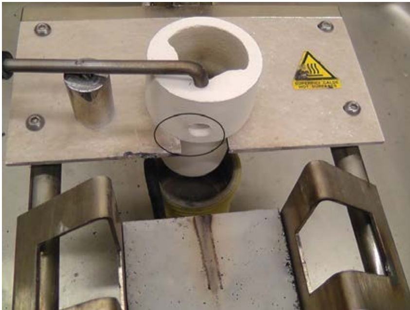
Figure 12: placing the crucible in the plate
